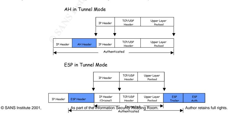
In Tunnel Mode, the whole packet is processed including the IP header. Original IP source and destination addresses and other header components are protected by AH or ESP, and a new IP header is inserted into the packet. The new IP source and destination addresses typically are those of the gateways. Based on the transformation method used, (AH or ESP), the whole packet is either authenticated, encrypted or both.
